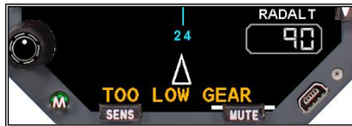
Figure 7-3 Generic GPWS Mode 4 Alert
