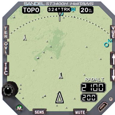
Figure 6-6 Minimized Obstacles in TOPO Display
