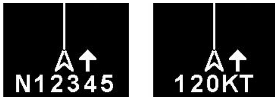
Figure 9-7 Aircraft ID and Ground Speed Display
