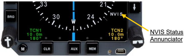
Figure 3-10 NVIS Status Annunciator
