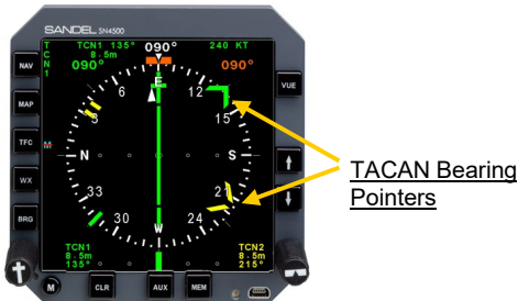
Figure 4-11 TACAN Bearing Pointers
