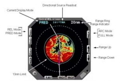
In PRED mode a red cell will always produce an FLTA alert when close enough to and on the aircraft's flight path. A yellow cell *may* produce an alert if it meets the alerting criteria; the alerting criteria are lower than the color coding criteria by a few hundred feet. For this reason not every cell colored "yellow" will produce an alert. A green or black cell will never cause an alert.
