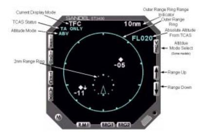
The traffic display mode is accessed by pressing the [TFC] button. If there is a Traffic Advisory alert and the aircraft is not on the ground, then the traffic display mode will be automatically selected.
