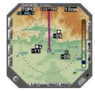
Traffic will be overlaid on terrain when in REL, PRED, and TOPO display modes. The same symbology is used as when the TFC display mode is chosen. *Traffic is always shown relative to the nose of the aircraft – where you would see it if you looked out the window.*
