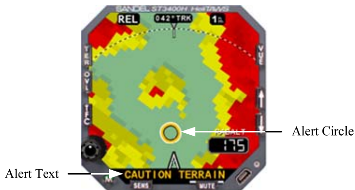
Figure 6-1 “CAUTION TERRAIN” Annunciation
