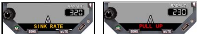
Figure 7-1 GPWS Mode 1 Alerts
