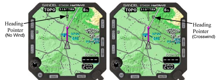
Figure 5-15 Heading Pointer – FULL View
