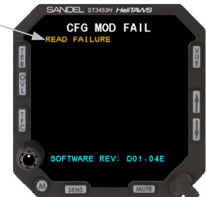
Figure 12-2 CM MOD FAIL Display
