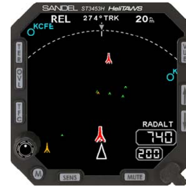
Figure 6-7 Obstacles in REL Display
