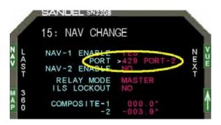
Repeat the above steps for NAV-2 ENABLE if dual 400W/500W units are interfaced to the SN3308.
