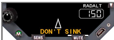
Figure 7-7 Offshore GPWS Mode 3A Alert
