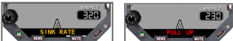
Figure 7-6 Offshore GPWS Mode 1 Alerts
