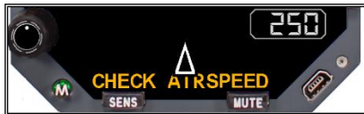
Figure 7-8 Offshore GPWS Mode 3B Alert
