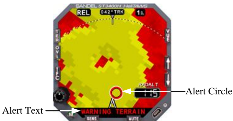
Figure 6-2 “WARNING TERRAIN” Annunciation
