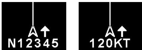
Figure 9-7 Aircraft ID and Ground Speed Display
