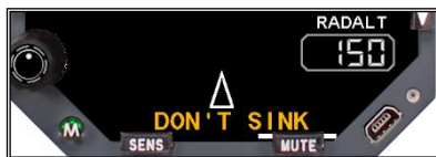
Figure 7-2 Generic GPWS Mode 3 Alert
