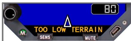
Figure 7-10 Offshore GPWS Mode 4B Alert
