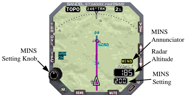
Figure 8-1 Radar Altimeter Functions
