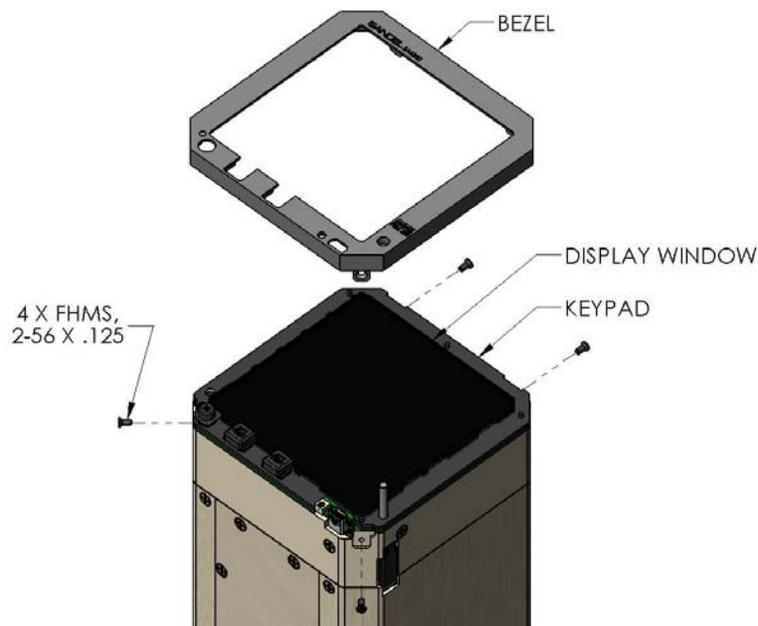
**Figure 5. Reinstall Bezel**
