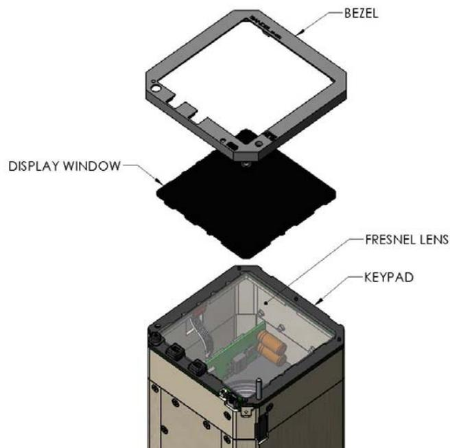
**Figure 3. Window removal**
