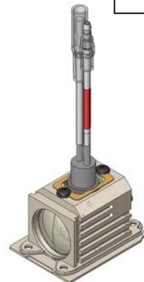
Fig. 7: Ensure lamp is fully seated into lamp housing. Torque pan head screw until snug.
