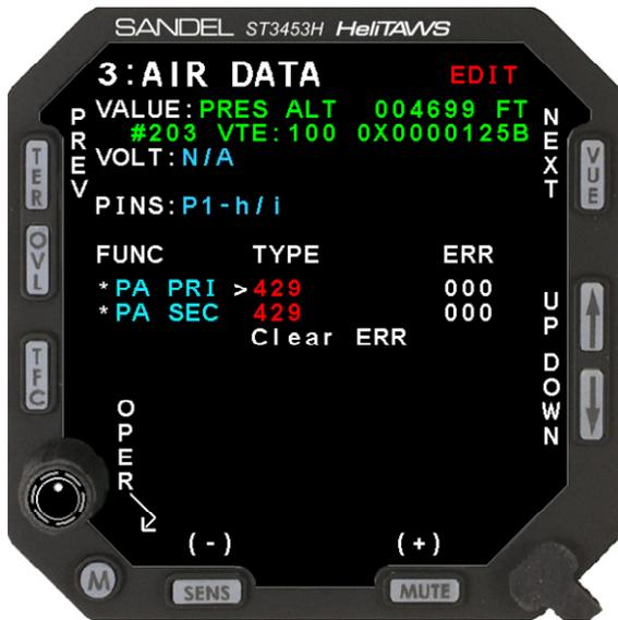
The Air Data page contains the setup information for the Airdata system. Use the [UP] or [DOWN] soft-keys to select a setup item. This will move the cursor to the appropriate line and display the current input data value, input voltage (if applicable) and pin-pairs of the selected signal.
