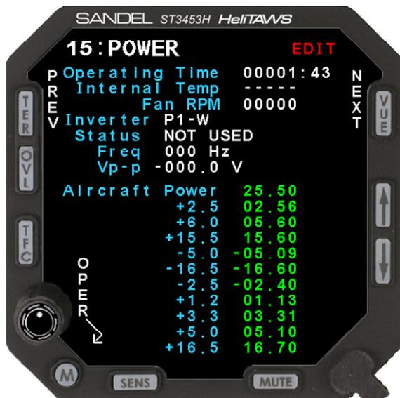
The Power maintenance page consists of readouts that monitor the unit’s internal environment and the unit’s power measurements for reference.
