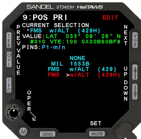
The POS PRI input is used for position data and flight plan data. The multiple-choice list allows the operator to specify the type of GPS/FMS connected to the POS PRI position ports. Select the desired receiver using the [UP]/[DOWN] soft-keys and use the [SET] soft-key to make the selection. Once a selection is made, the port configuration will be automatically made based on the selection chosen and data will appear in the data VALUE area.
