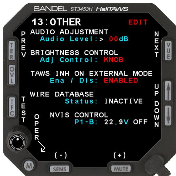
This page is used to allow the installer to specify the nominal and maximum audio levels for the low level audio output. The low level output acts as master gain. Initiate an audio level test by selecting the desired volume level and pressing the TEST soft-key. This may be used to show the result of changing the audio level adjustments.
