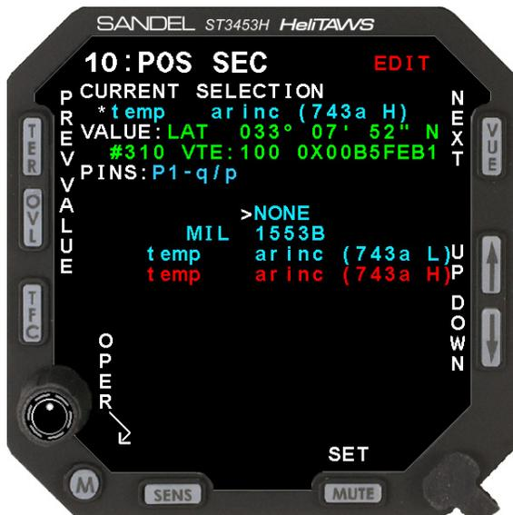
The POS SEC input is used for position data. The multiple-choice list allows the operator to specify the type of GPS/FMS connected to the POS SEC position ports. Select the desired receiver using the [UP]/[DOWN] soft-keys and use the [SET] soft-key to make the selection. Once a selection is made, the port configuration will be automatically made based on the selection chosen and data will appear in the data VALUE area.
