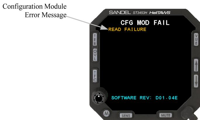
The user cannot exit this screen. If this screen appears, the unit is non-operational and must be serviced.
