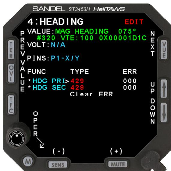
The HDG page contains the setup information for the HDG system. Use the [UP] or [DOWN] soft-keys to select a setup item. This will move the cursor to the appropriate line and display the current input data value, input voltage (if applicable) and pin-pairs of the selected signal.
