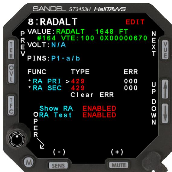
The Radalt page selects the configuration of Radar altimeter input. If no Radar altimeter is installed set configuration of RALT to NONE.
