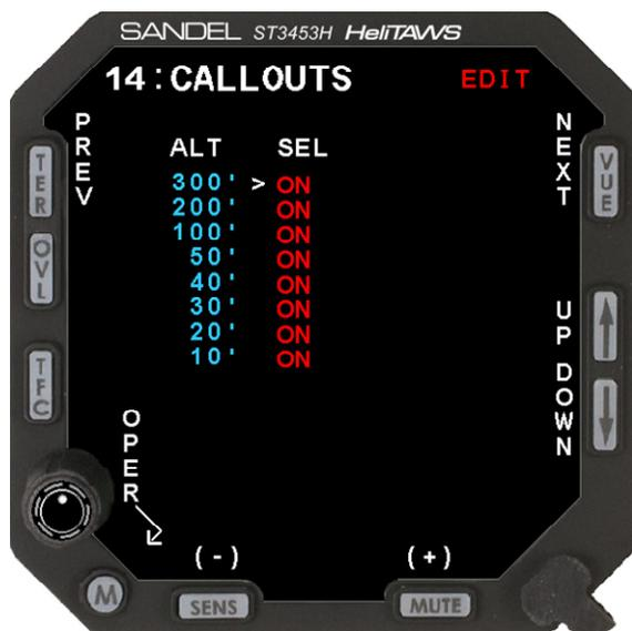
The Callouts page allows enabling Radar Altitude audio callouts. Use the [UP] or [DOWN] soft-keys to select a setup item, this will move the Cursor to the appropriate line. [+] and [-] select “ON” or “OFF for each callout.
