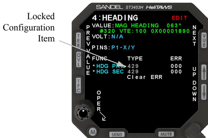
Once the Maintenance Menu is entered, press the [NEXT] or [PREV] soft-keys to cycle the MAINTENANCE MENU pages. To jump to a specific page, from the INDEX page, press the [UP] or [DOWN] soft-key or rotate the knob to move the cursor. Press the [SELECT] soft-key to jump to that page. On some menus additional soft-key legends will appear as prompts.
