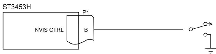
NVIS CONTROL/Discrete - Active High (OPTIONAL)
