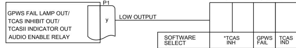
\*TCAS INH selection may be used to drive a 'TAWS audio enable' relay if desired. See 82050-10, Sheet 1
