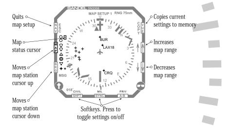
Map setup allows you to change the scratchpad memory S by adding or deleting items from the map category by category. The two buttons located next to the map status are used to move the map status cursor up and down, selecting the different map setup items you want to change.
