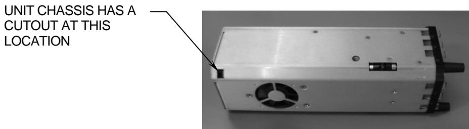
**STEP A** Reinstall the SN3308. Tighten the bottom right mounting screw in the panel. Insert a 7/64" Allen key into the lower left mounting hole approximately 3/4" and you will engage a jackscrew. Rotate the jackscrew fully clockwise until finger tight. Insert the SN3308 in the clamp tray, continue rotating the jackscrew counter-clockwise until the SN3308 is fully engaged in the tray connectors. Reinstall the single size 8-32 screw in the lower-left of the SN3308. Tighten the two upper screws.
