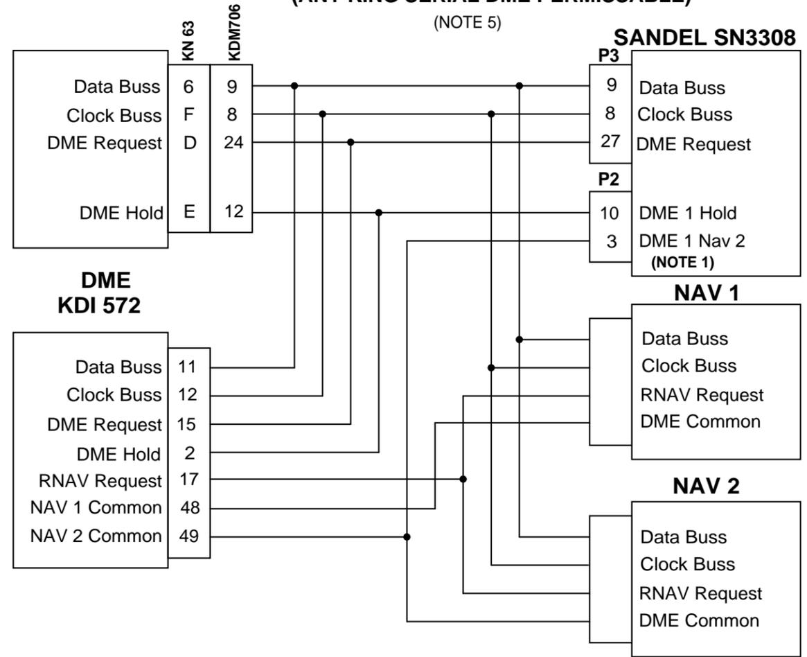
**SINGLE KING SERIAL DIGITAL DME WITH SELF CONTAINED CONTROLLER
