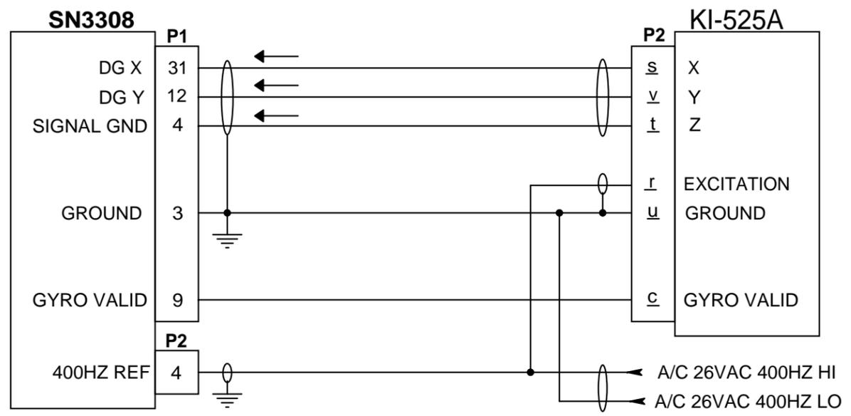
**USING KMT-112 FLUX GATE WITH 26VAC INVERTER
