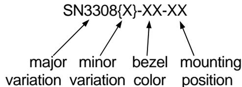
The “**L**”, “**C**”, and “**R**” variants signify the position in which the unit is to be mounted within one of the three predominate locations, i.e. Left instrument panel, Center panel, and Right instrument panel. The viewing properties of the display are optimized by the correct selection of part number.
