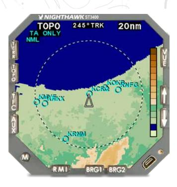
The TSO'd, FAA-approved Class A and Class B TAWS solution, the ST3400 TAWS/RMI is the standard in TAWS performance. Reliable, affordable and easy to install, the ST3400 is a compact, self-contained unit that enhances pilot situational awareness as it helps avoid the problem of controlled flight into terrain (CFIT).
